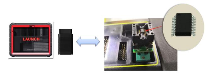
**Connection method 3**: After removing the ECU from the car, connect the anti-theft ECU pin to the DIY slot of the immobilizer programmer through the cable to realize the data interaction between the anti-theft ECU and the diagnostic host.
