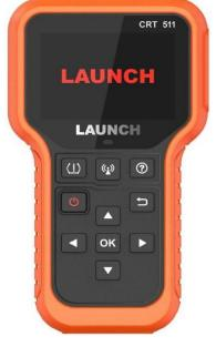
CRT-511 is a professional TPMS diagnostic tool that integrates TPMS sensor activation, reading, learning and programming. It can activate and read tyre pressure sensor information through radio frequency. It uses the OBD interface to reset the TPMS modules, programming the sensor by receiving a frequency of 433 MHz.
